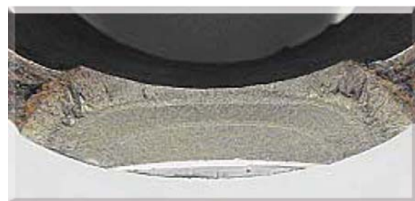
Fig. 19: Typical fatigue fracture surface of pipe (1x1)
